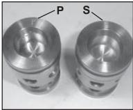
5. When reassembling: The suction valve seat (51C) is 1mm smaller in diameter than the discharge valve seat (52C). Suction valve seats are marked "S" and always have to be installed first. Discharge valve seats are marked "P" and are always tobe installed on top of suction valve. Plugs (58) are to be tensioned down evenly with screws (58C) and crosswise at 156 ft-lbs. (210 NM).
